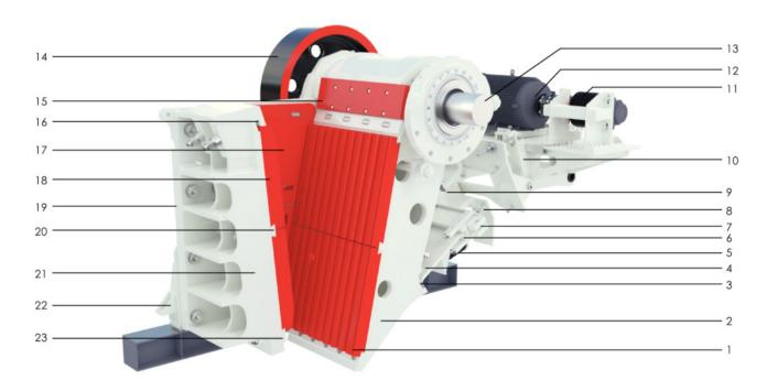
1.动颚板 movable jaw plate 2.动颚 movable jaw assembly 3.肘板垫 toggle plate seat 4.肘 板 toggle plate 5.弹 黉 spring 6.调整座 adjusting base 7.调整楔块 adjusting wedge 8.弹簧护板 spring guard plate 9.后墙 rear frame 10.电机座 motor seat 11.电机轮 motor pulley 12.电机 motor 13.偏心轴 eccentric shaft 14.飞轮 flywheel 15.动颚护板 movable jaw guard plate 16.上楔块 upper pressing wedge 17.边护板 side guard plate 18.定颚板 fixed jaw plate 19.侧墙板 side frame 20.中间压铁 middle pressing wedge 21.前墙 front frame 22.支架 supporting base 23.颚板下挡块 bottom wedge
